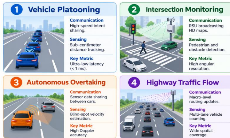
Figure 13.1 ISAC Performance Requirements in Smart Transportation [6].
